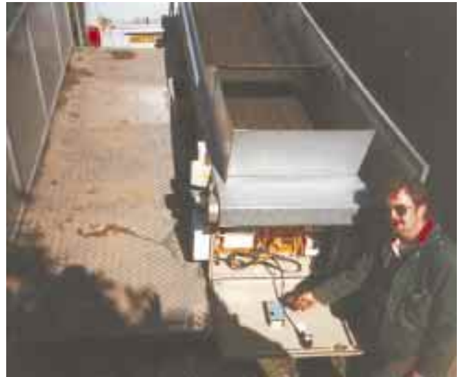
Above: The feed end of the conveyor belt. Phil Evans shows the inside of the opened power panel.
